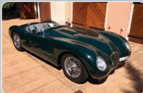
1951 Jaguar C Type Replica British Racing Green with Green leather seats, built by Nostalgia Cars UK, Fibreglass body, space frame chassis with Aluminium panels, 4.2L XJ6 Motor, 5 speed manual gearbox, disc brakes. POA
